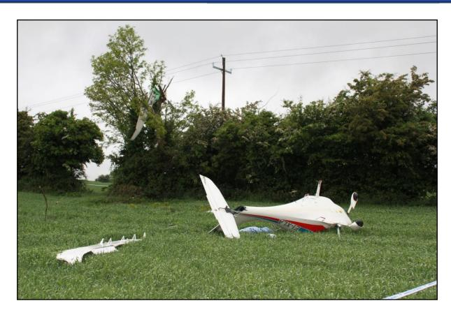
**Photo No. 1:** Final resting position of EI-XLA with bent insulator on top of utility pole and wing embedded in tree.
